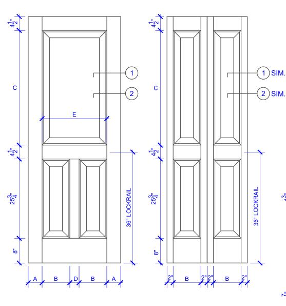
**DOOR COMPONENT SIZES TOP** STILE **PANEL MIDRAIL PANEL PANEL WIDTH WIDTH WIDTH WIDTH HEIGHT** "A" "B" "D" "E" **DOOR WIDTH** "C" 2-0 THRU 2-4 **VARIES VARIES** 2" **VARIES** 4-1/2" **VARIES VARIES** 3" **VARIES** 2-6 THRU 4-0 NOTES:
