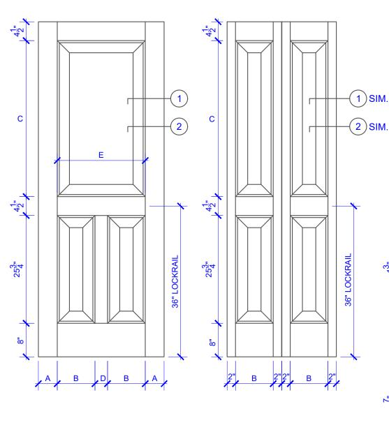
STILE **PANEL MIDRAIL PANEL PANEL WIDTH WIDTH WIDTH WIDTH HEIGHT** "A" "B" "D" "E" **DOOR WIDTH** "C" 2-0 THRU 2-4 **VARIES VARIES** 2" **VARIES** 4-1/2" **VARIES VARIES** 3" **VARIES** 2-6 THRU 4-0 NOTES: 1. BIFOLD LEAF WIDTHS 10-11/16"-24" WILL HAVE 2" WIDE STILES.
