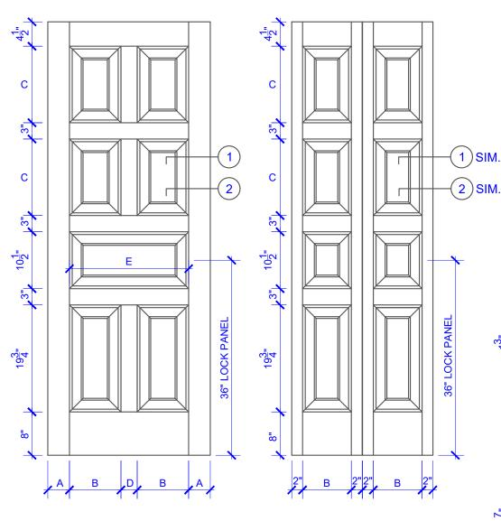
**DOOR COMPONENT SIZES** STILE **PANEL MIDRAIL PANEL PANEL WIDTH WIDTH WIDTH WIDTH HEIGHT** "A" "B" "D" "E" **DOOR WIDTH** "C" 2-0 THRU 2-4 **VARIES VARIES** 2" **VARIES** 4-1/2" **VARIES VARIES** 3" **VARIES** 2-6 THRU 4-0
